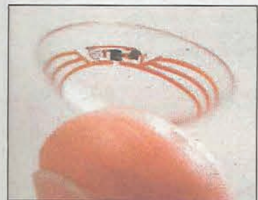
Designed to help diabetics: Google X Lab's smart contact lens measures glucose in tears to avoid pinprick tests
